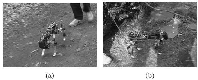
Fig. 23 Photos of walking of Tekken2 on natural ground. The cable is just to prevent Tekken2 from damage in case of emergency, and usually slack. The average walking speed was approx. 0.7 [m/s]
